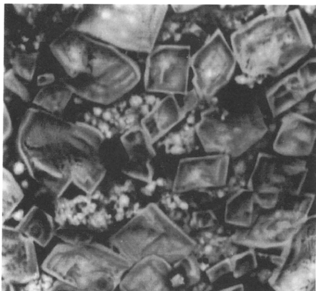
Fig. 4. Secondary-electron micrograph of the surface of a grid/corrosion layer sample from a formed Pb–Ca positive plate. Bar length: 10 \mu\text{m} .
